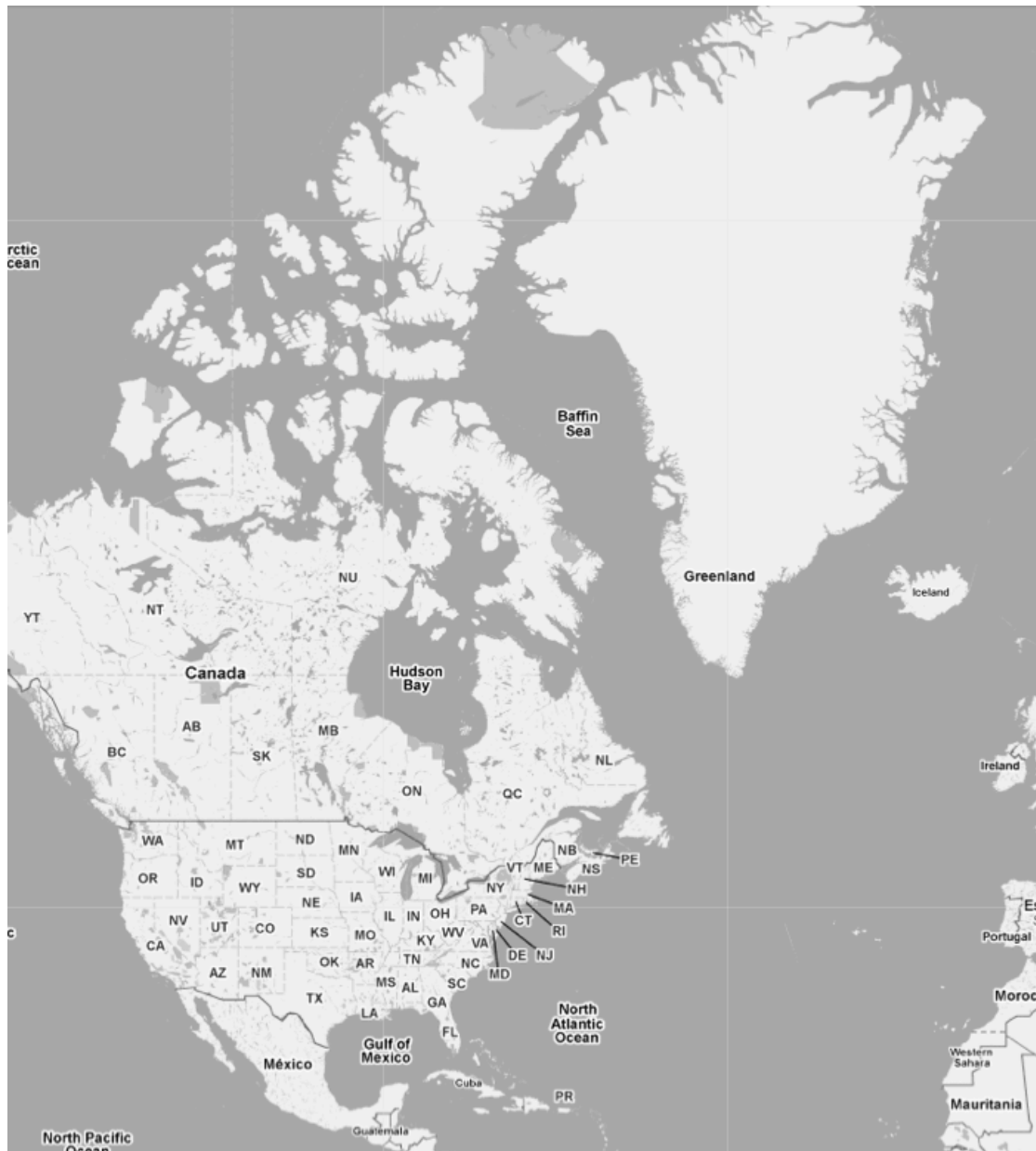
FIGURE 3: In this screenshot from Google Maps, Greenland appears as large as Canada due to the area distortions inherent to the Mercator projection. Had Google chosen an equal-area projection, Greenland's area would have been accurately depicted as being approximately that of Mexico.
